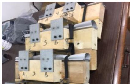
The band marks were predominately noticed on doors that had been through high temperatures, up to 140°F, between manufacturing and installation. Torsion began to investigate solutions that would reduce the marks and have a minimal cost impact and minimal change to low
